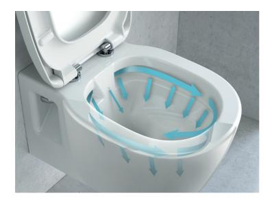
The water gushes through the 2 bigger lateral flushing orifices on the back of the functional area and along a visible flushing route that follows the outer perimeter on the top of the bowl. The smaller orifice in the middle sprays the bowl area over the syphon.
